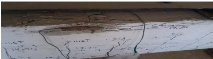
FIGURE31: COMPRESSION FAILURE FOR NA BEAM
