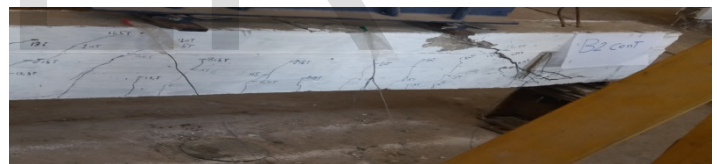
FIGURE28: CRACK DISTRIBUTION FORNAC1 BEAM
